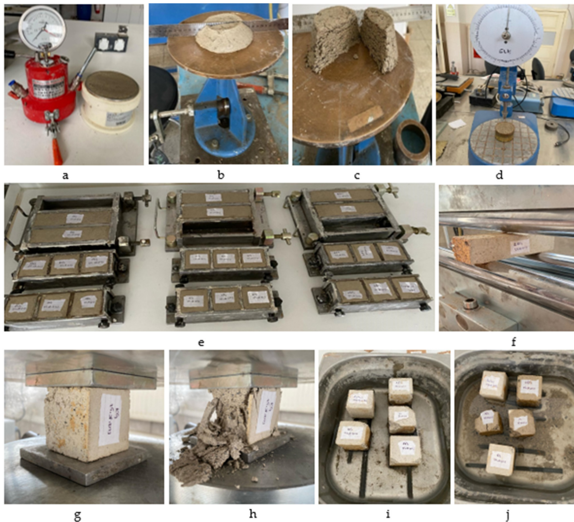
Figure 2. Tests applied: (a) Air content determination; (b,c) Flow table; (d) Fall cone; (e) Sample preparation; (f) Flexural strength; (g,h) Compressive strength; and (i,j) Capillary water absorption.
