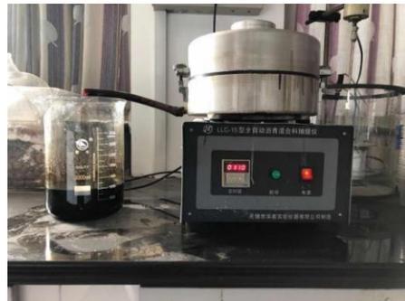
Figure 2. Centrifugal extraction test chart.
