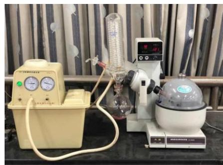
Figure 3. Rotational evaporation test diagram.
