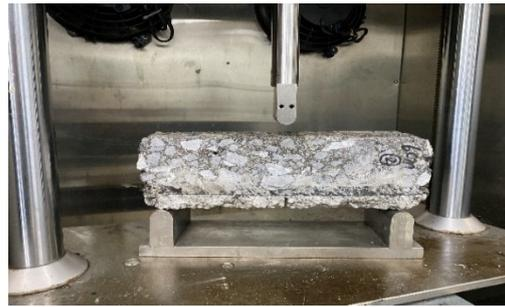
Figure 10. Three-point bending test loading die.
