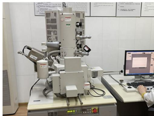
**Figure 18.** Scanning electron microscope.
