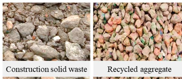
**Figure 2.** Recycled construction-solid-waste aggregate.
