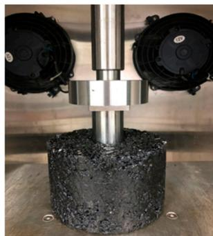
**Figure 5.** Loading diagram of uniaxial penetration test.
