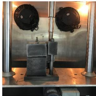
**Figure 7.** Loading mode of interlaminar shear test.
