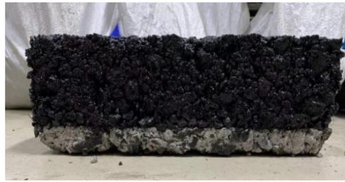
**Figure 4.** Basalt fiber rubber asphalt stress absorption layer specimen.
