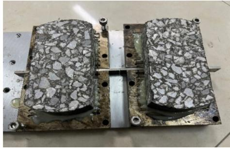
Figure 14. Epoxy resin fixed test piece.
