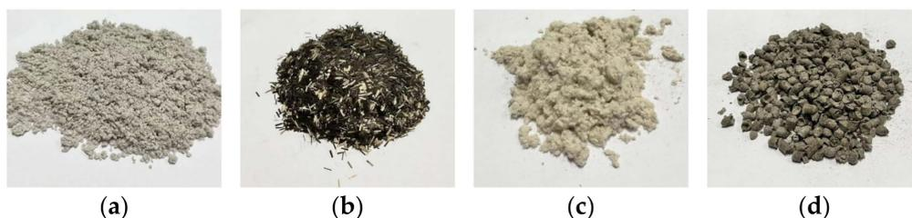
**Figure 1.** Morphologies of fiber additives. (a) Flocculent basalt fiber; (b) chopped basalt fiber; (c) flocculent lignin fiber; (d) granular lignin fiber.
