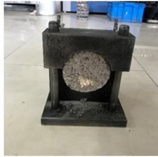
**Figure 6.** Fixing method of interlaminar shear test mold.
