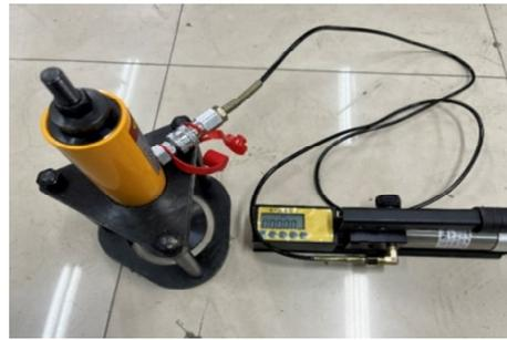
**Figure 8.** XH-15 T subgrade and pavement adhesion performance tester.
