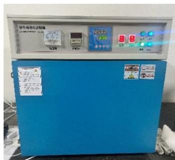
**Figure 7.** UV aging chamber.
