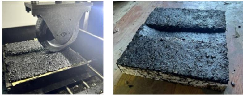
Figure 9. Rutting depth of the original pavement.
