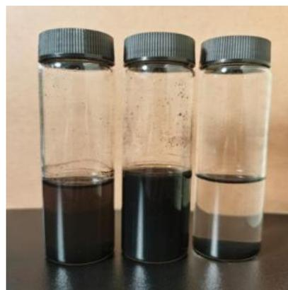
Figure 8. (a) Zeta–pH curves of carbon black and CMC-AMPS-AM. (b) Addition of 37.5% dispersant to carbon black at different pH (right pH = 12, middle pH = 7, and left pH = 2). Natural settling effect can be seen for the right vial with high pH.
