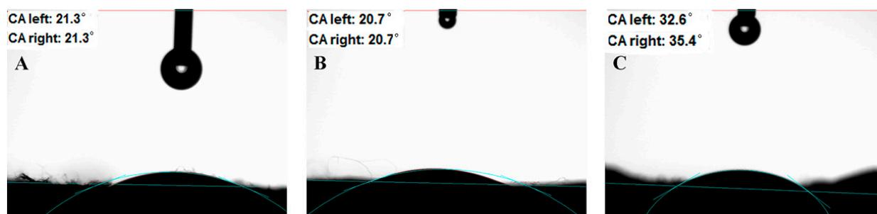
**Figure 8.** Water contact angle images: (A) PAN/PVP; (B) PAN/PVP/P25-0.2; (C) PAN/P25-3.
