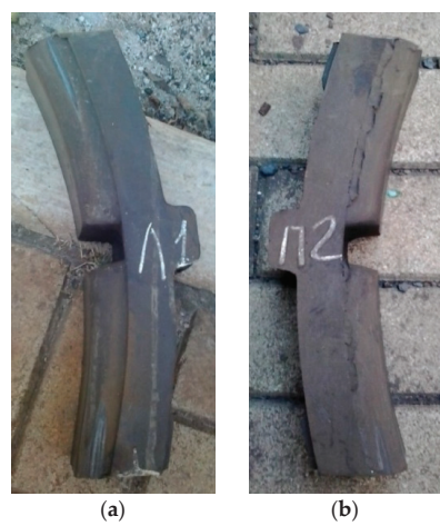
Figure 3. A sample a composite brake pad with uniform wear with regard to the thickness: (a) the first brake pad in the running direction (marked as 11); (b) the second brake pad in the running direction (marked as 12).
