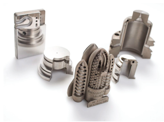
Figure 3. Examples of conformal cooling channel [16].
