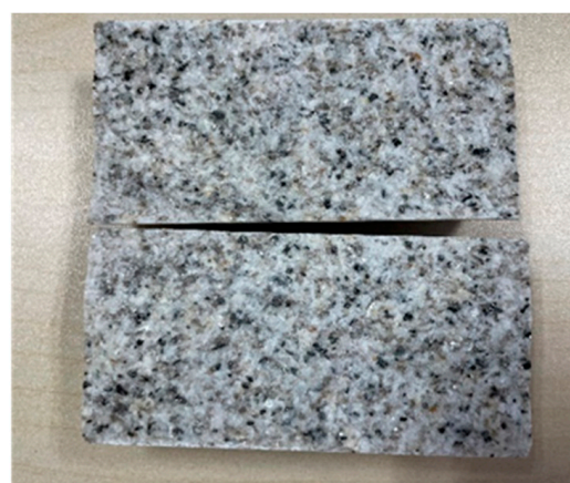
A complete fracture (core completely cracked)
