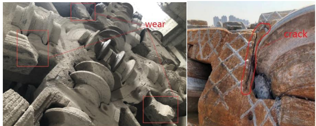
Figure 2. Failed cutterhead of a shield machine.
