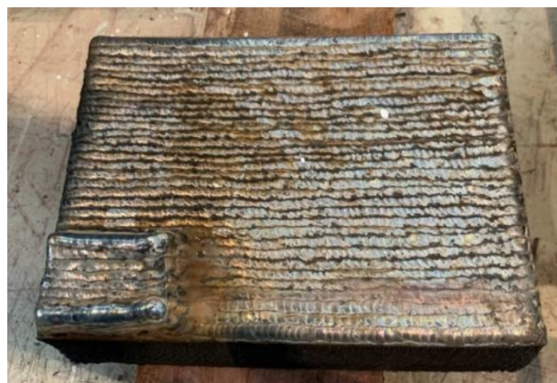
Figure 2. Plain plate welded by manual TIG welding technique.
