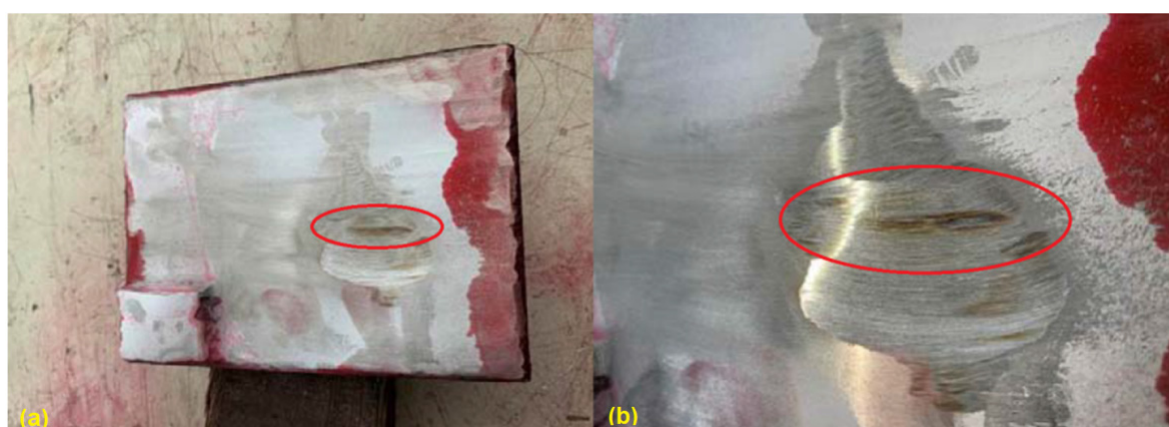
Figure 3. Appearance of the welded plate after liquid penetrate test (a) and cracks (b).
