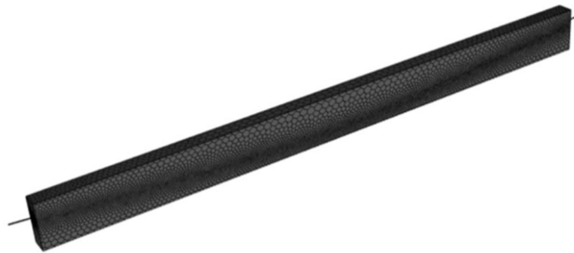
Figure 12. Electrothermal model for controllable bonded reinforcement.
