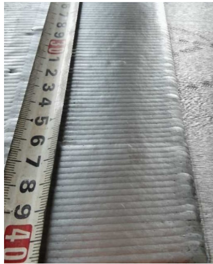
Figure 6. Appearance of first batch of laser weld overlay.
