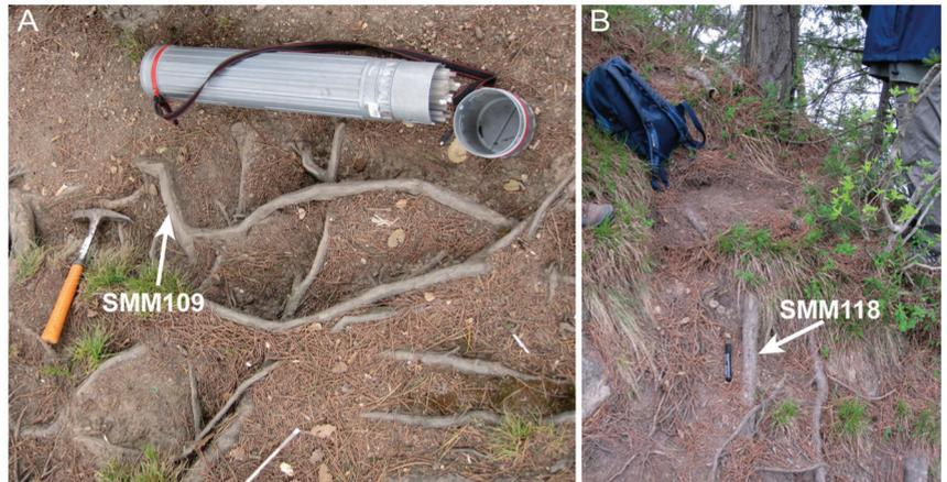
**Figure 2.** Field photos of exhumed roots. (A) A network of exhumed roots probably belonging to multiple trees. The position of sample SMM109 is shown. (B) Exhumed roots parallel to the slope. The position of sample SMM118 is shown.
