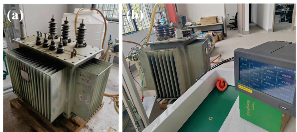
Figure 5. The waste transformer and the full oil recovery test. (a) The waste transformation. (b) The full oil recovery test.
