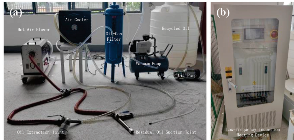
Figure 3. Full recovery system for waste transformer insulating oil and low-frequency induction heating device. (a) Full recovery system. (b) Low-frequency induction heating device.
