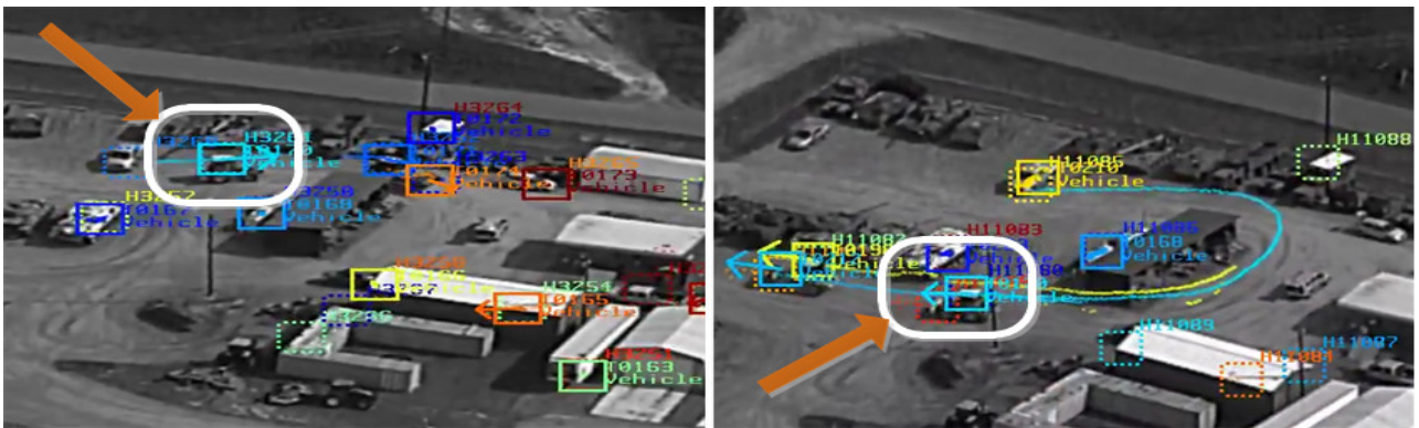
Figure 8. Illustration of an exemplar target track (from the ApHill VIRAT aerial dataset) being matched to the proper activity pattern model (a u-turn in this example) learned using the training data generated by the proposed multi-source association approach.
