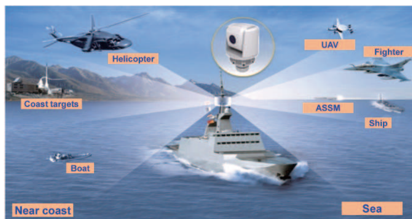
Figure 1. Operational concept of sea-based infrared search and track (IRST).
