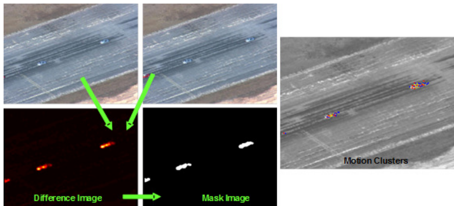
Figure 2. Video-indexed by voice annotations (VIVA)’s movement detection module. First, registered frames ( top left ) are differenced to produce a change detection image ( lower right ). That image is thresholded to detect changing pixels. Point correspondences within those detection pixels are established between the two frames and used to generate motion clusters ( right ).
