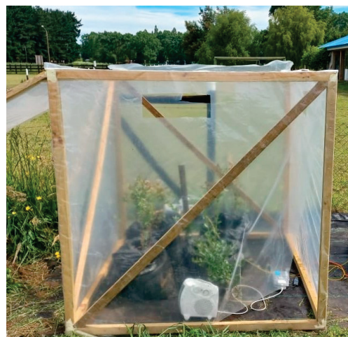
Figure 7. High-temperature chamber covered with transparent polyethylene (100 \mu\text{m} thick).
