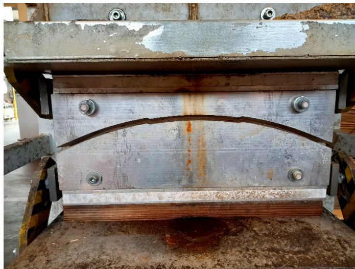
Figure 2. Molded plywood in the molded press during the pressing process.
