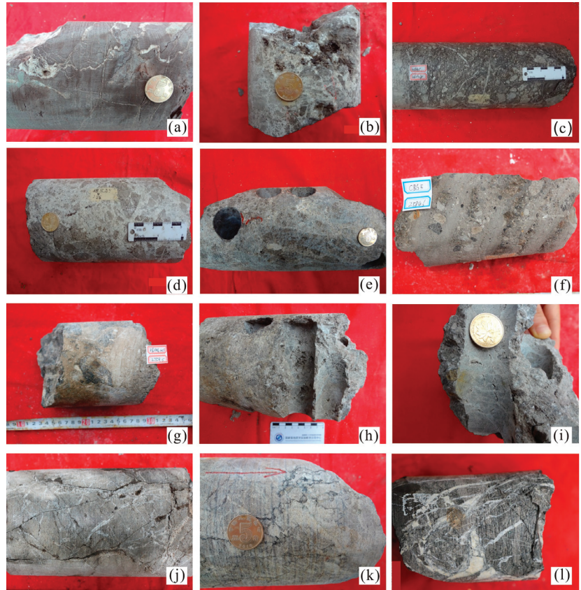
Figure 5. Core characteristics of Yeli-Liangjiashan Formation in Chengdao-Zhuanghai buried hill. (a) Well CBG100, 2562 m, granular (fine crystalline) dolomite, the high angle crack is connected with the dissolved pore; (b) Well CBG5, 2586 m, dolomitic breccia, dissolved pores developed, partially filled with calcite; (c) Well CBG5, 2602 m, the dolomitic breccia with good roundness is arranged in a directional manner; (d) Well CBG5, 2585.4 m, dolomitic breccia, high degree of calcite vein filling; (e) Well CB302, 4002.16 m, intergranular dolomite filled with calcite; (f) Well CBG5, 2584.6 m, granular dolomite, subrounded breccia, layered dissolved pores are developed; (g) Well CB403, 2759.5 m, the dolomitic karst breccia is interspersed with percolating sand; (h) Well CB302, 4001.26 m, limy karst breccia with dissolved pores developed and a small part filled with soil; (i) Well CB302, 4001.86 m, limy karst breccia with unfilled pore development; (j) Well CBG5, 2601.5 m, limy dolomite cracks are developed, and the cracks are filled with mud; (k) Well CBG100, 2560.47 m, dolomite limestone, high angle crack development; (l) Well CB244, 2921.27 m, granular (fine crystalline) dolomite, network cracks filled with calcite veins.
