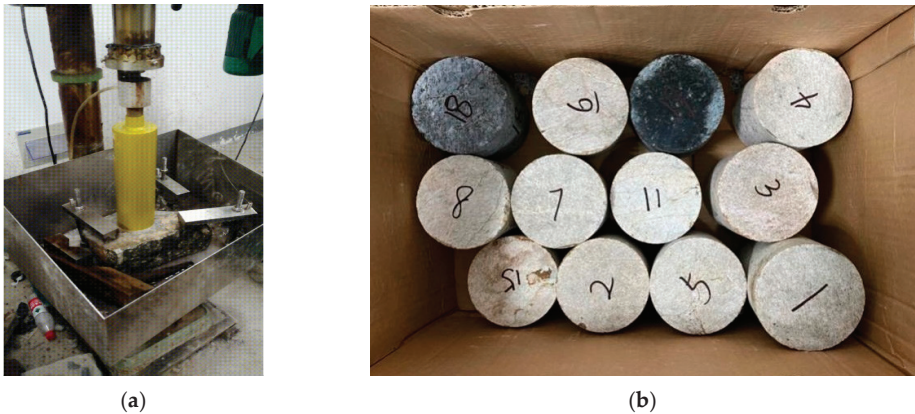
Figure 10. Full-diameter core drilling schematic diagram. (a) Drilling the operating table; (b) Core drilling finished product.
