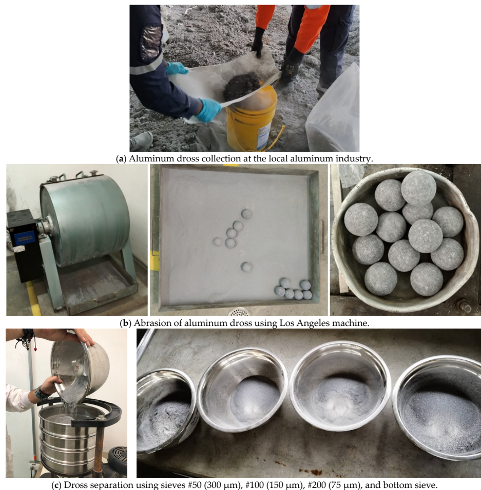
Figure 3. Aluminum dross collection and inactivation processes.
