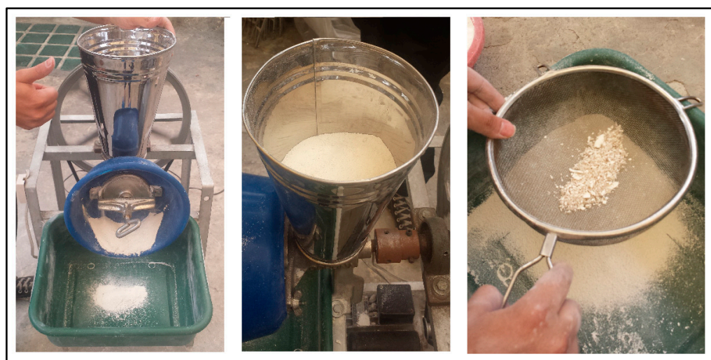
Figure 1. Detail of waste uniformization and homogenization.
