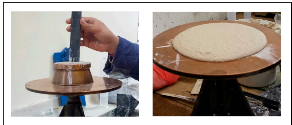
Figure 3. Details of the flow test.
