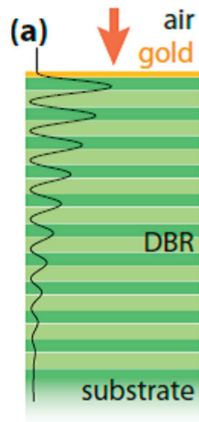
Figure 6. Schematic view of the Tamm structure: a GaAs/AlAs DBR with a gold film. The letter (a) indicates the pattern of light intensity distribution in the structure. Reprinted with permission from [29] © Optical Society of America.
