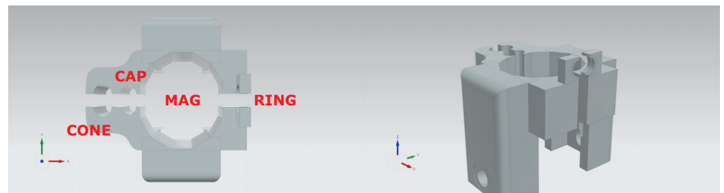
Figure 5. The left view is a top-down perspective highlighting the central decagonal (10-sided) hole for gripping the MAG. Moving to the right, there is a hole for the CAP and a conical hole for gripping the CONE.
