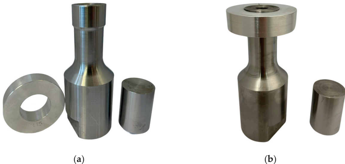
Figure 11. (a) Specimens before joining and (b) press-fit connection after the joining process.
