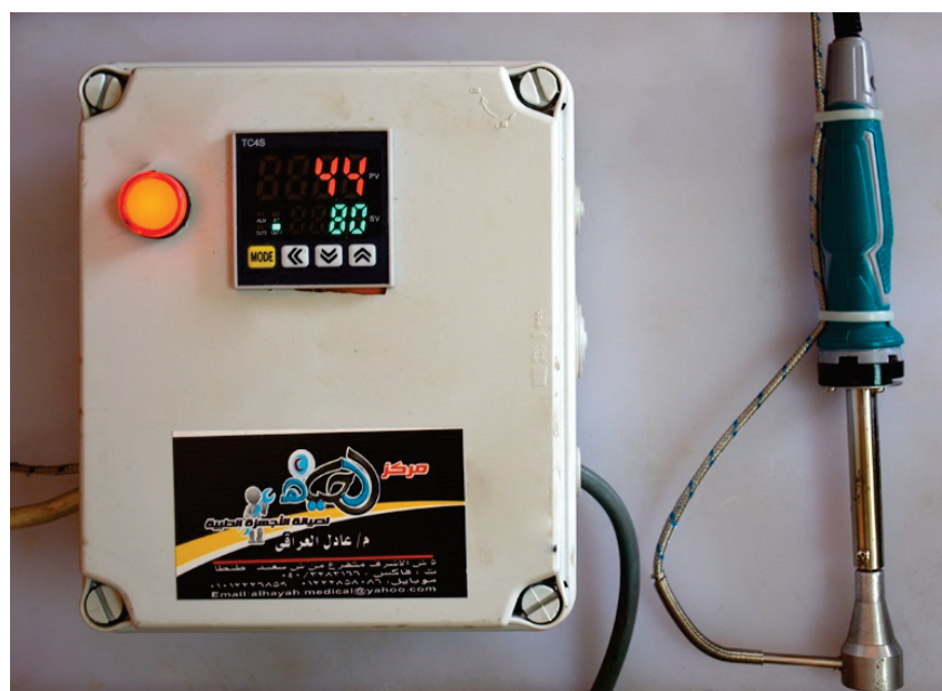
Figure 2. Adjustable electrical aluminum stamp for induction of thermal burn-wounds.
