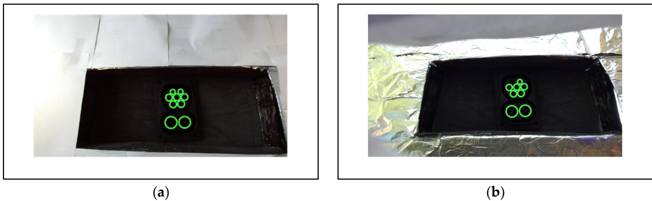
Figure 17. Results of the comparison with Circular Hough Transform: (a) Correct detection, (b) incomplete detection.
