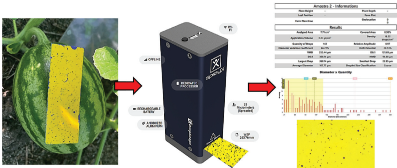
Figure 5. Wireless system (DropScope®; SprayX, São Carlos, Brazil) used for scanning the water-sensitive papers.
