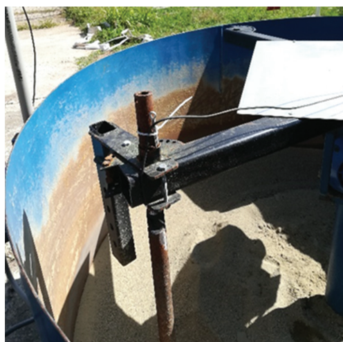
Figure 8. Experimental stand for testing chisel-type knives. Close-up view of the chisel knife on the experimental stand.
