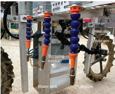
Figure 13. The external appearance and the internal configuration of the spray nozzle.
