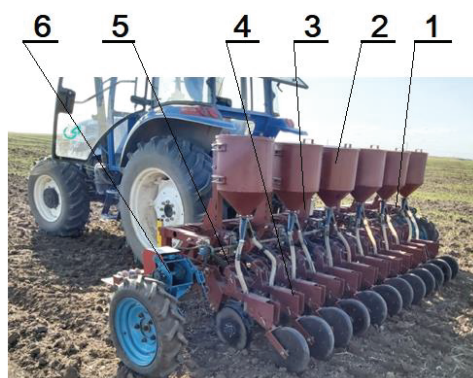
Figure 1. The view of the experimental seeder for sowing non-flowing grass seeds: 1—frame; 2—seed box with sowing machines; 3—hinged device; 4—sowing section; 5—seeding machine drive; 6—running gear.
