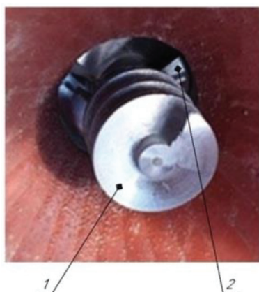
Figure 3. The image of a sowing unit for non-flowing grass seeds: 1—rotator; 2—blade supercharger.
