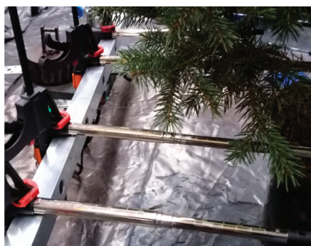
Figure 3. Example of the method of mounting anemometers on the tripod for placement in the tree crown.
