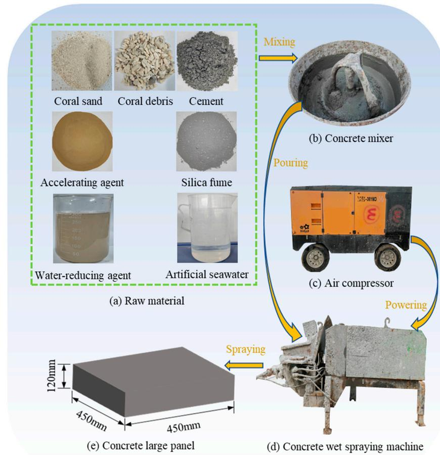
Figure 3. Schematic of the large-panel specimen-making process.
