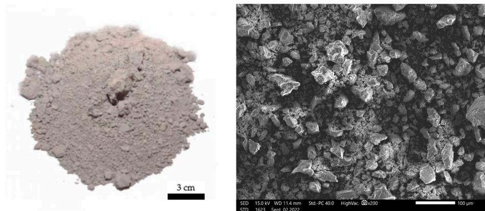
**Figure 3.** SEM microstructure of the fly ash used in the study and visualization of the form in which it was used.
