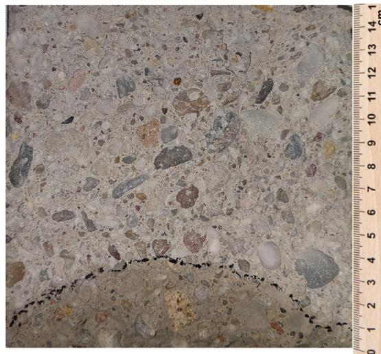
Figure 10. View of the concrete sample after the depth of penetration test.
