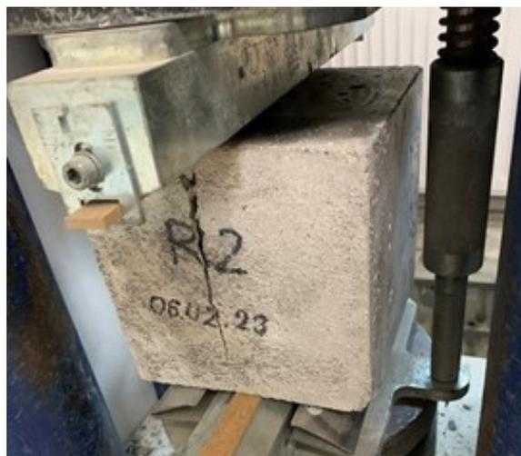
Figure 5. Splitting a sample after a water penetration test.
