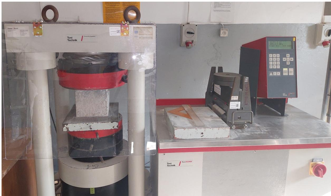
**Figure 3.** View of stand for compressive strength testing.
