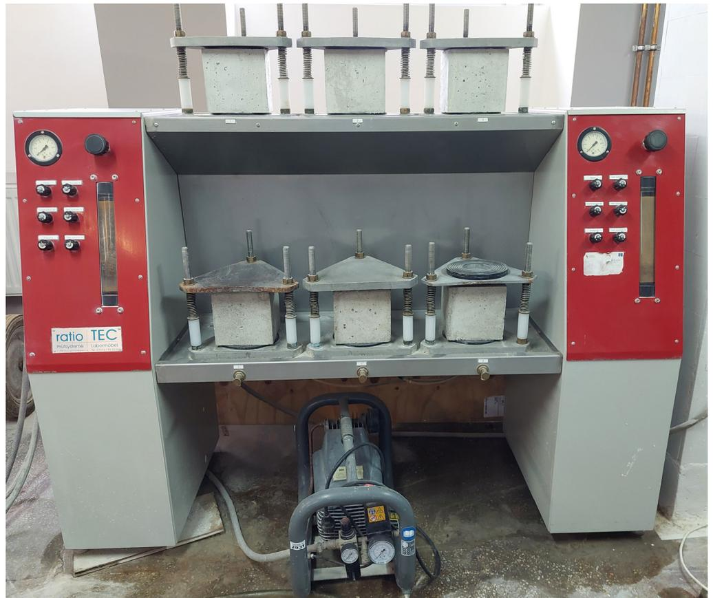
Figure 4. View of samples during water permeability test.
