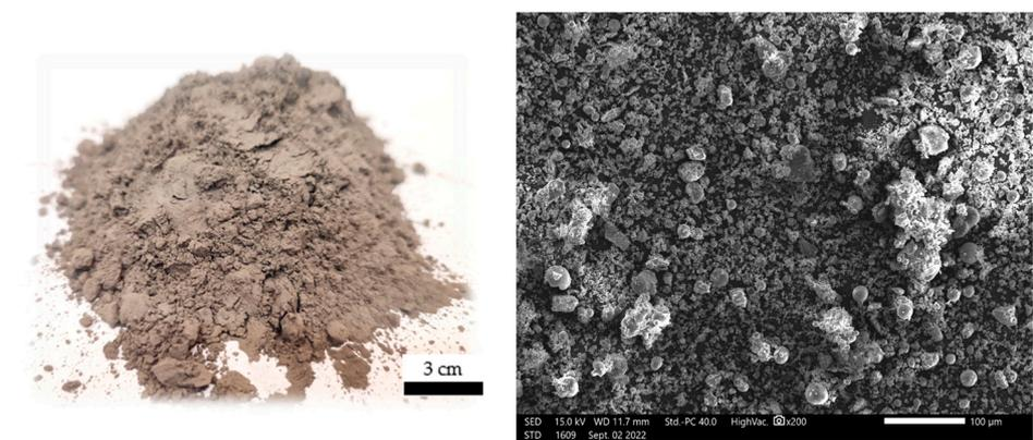
**Figure 4.** SEM microstructure of the basalt (basalt powder) used in the study and visualization of the form in which it was used.
