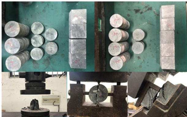
Figure 3. Coal rock body mechanical properties are part of the standard rock sample test damage map.
