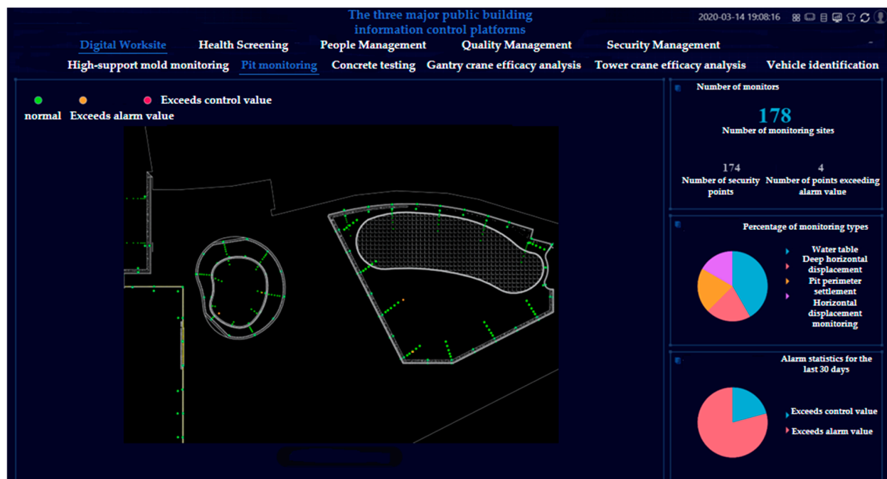
Figure 6. Twin platform for foundation pit safety monitoring.
