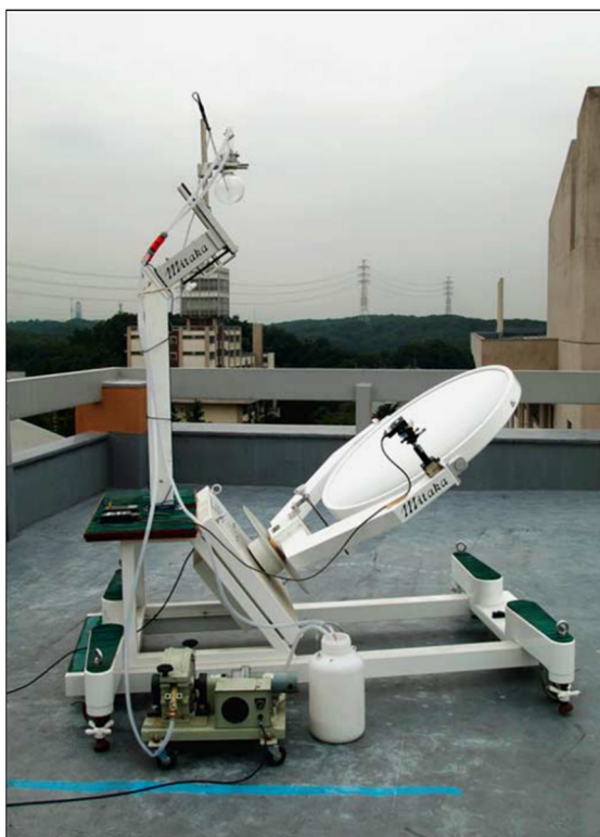
Figure 5. Parabolic dish collector for photocatalytic degradation of detergent (adapted with permission from ref. [82]. Copyright 2004 Elsevier B.V.).
