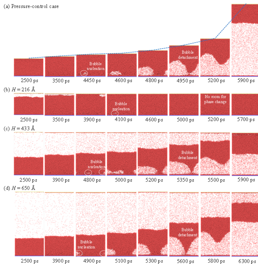
Figure 4. Snapshots of nucleate boiling of liquid argon on smooth surfaces with (a) pressure control method, (b) simulation box height H = 216 Å, (c) H = 433 Å, and (d) H = 650 Å. Bubble nucleation and detachment during the boiling process are also marked correspondingly.
