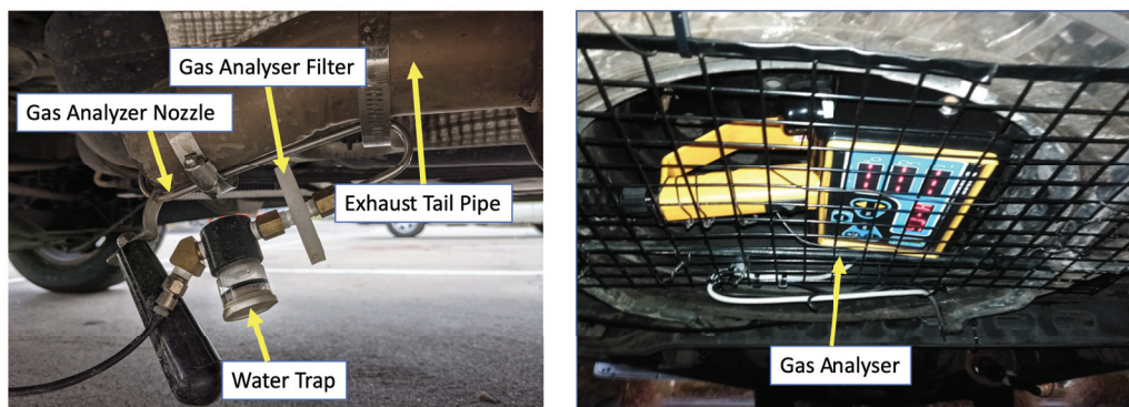
Figure 4. Gas analyser installed under the van.
