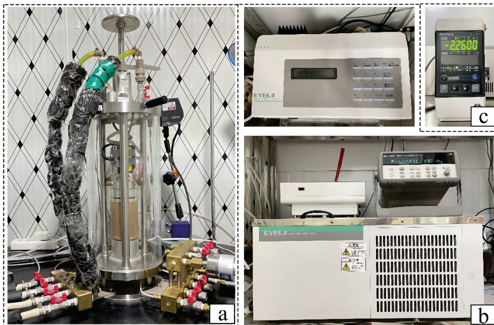
Figure 3. The main instrument used in the experiment: (a) Precision frost heave triaxial instrument; (b) Constant temperature water tank; (c) Data collector.
