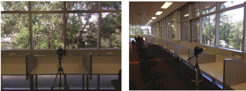
Figure 4. Example of taking high-dynamic-range (HDR) photos at each workstation.
