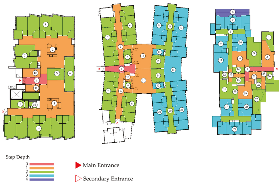
Figure 8. Relative depth analysis layout: Facility A (left), Facility B (middle), and Facility C (right).
