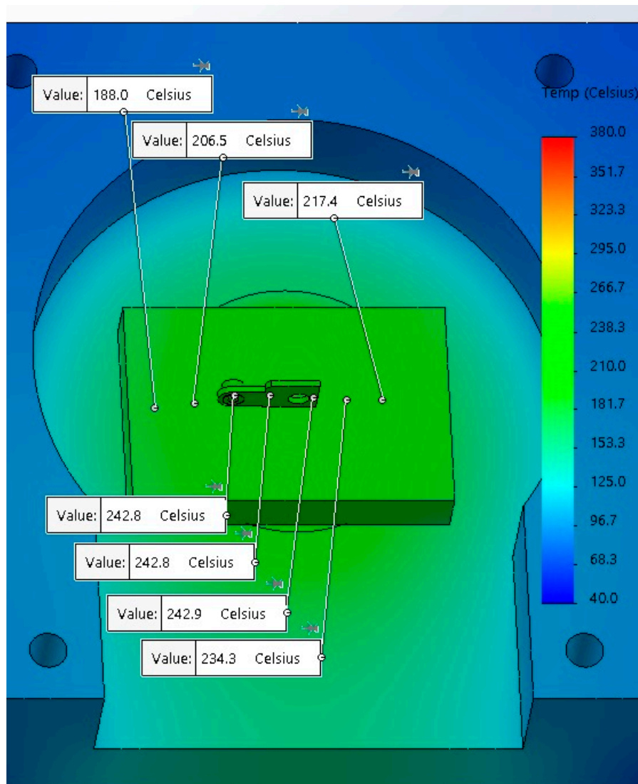
Figure 4. Temperature distribution during microwave soldering process.
