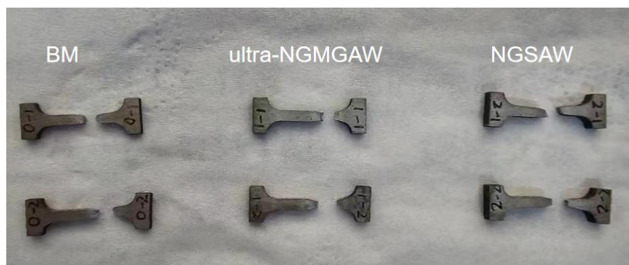
Figure 10. Tensile specimen after fracture.
