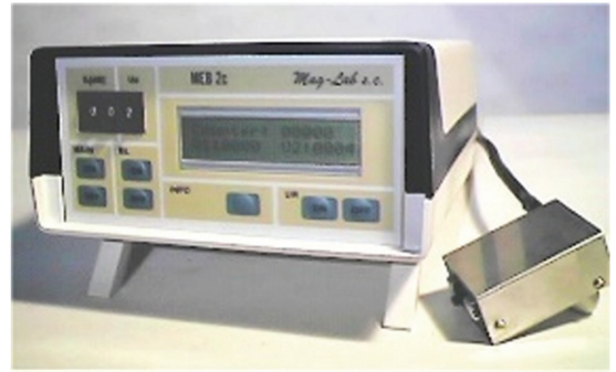
Figure 3. The MEB-2c probe used for the initial determination of magnetic properties. The schematic of the sensor (left). The actual probe with the electronics (right).
