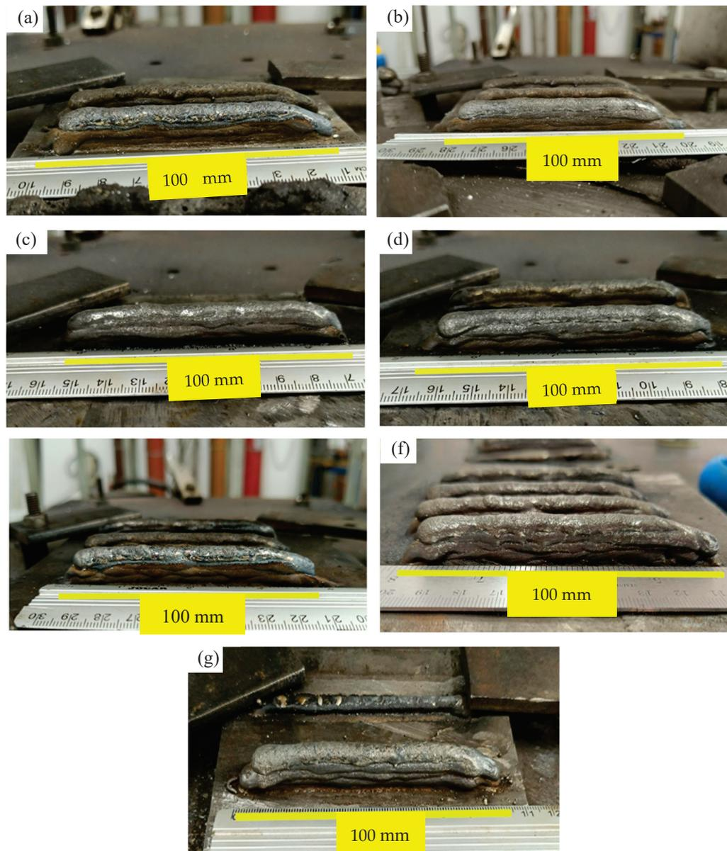
**Figure 2.** Fabricated walls: (a) W2, (b) W3, (c) W4, (d) W5, (e) W6, (f) W7, and (g) W1.
