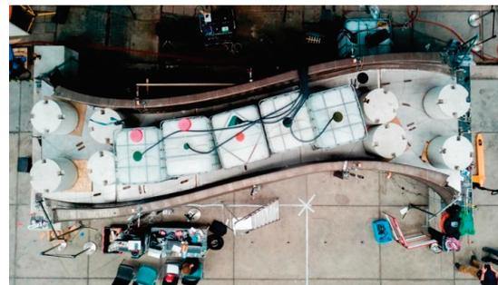
**Figure 18.** Load tests of MX3D bridge at the University of Twente. Reprinted with permission from ref. [79]. Copyright 2020 Elsevier Ltd. Reprinted from ref. [122].
