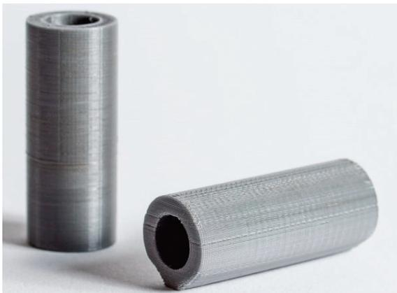
**Figure 14.** Two identical pieces printed in vertical (**left**) and horizontal (**right**) direction. Reprinted from ref. [98].
