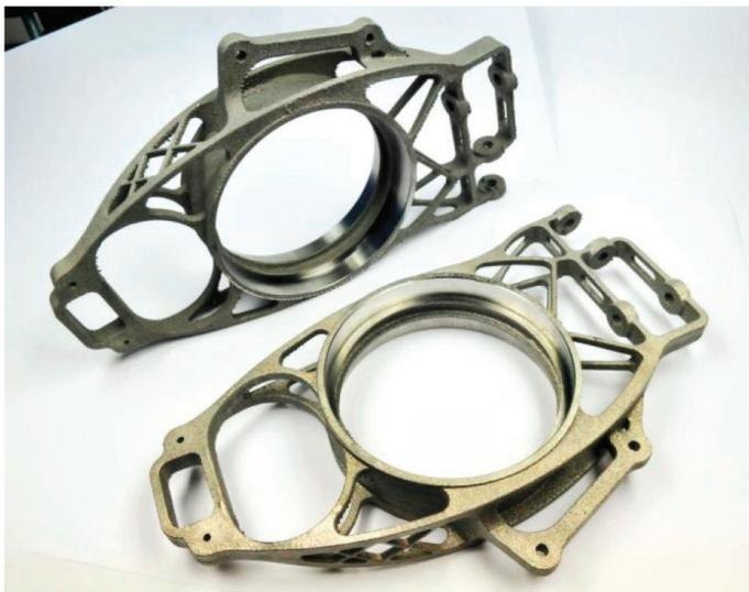
**Figure 24.** Optimized suspension uprights. Reprinted with permission from ref. [138]. Copyright 2017 Elsevier Ltd.
