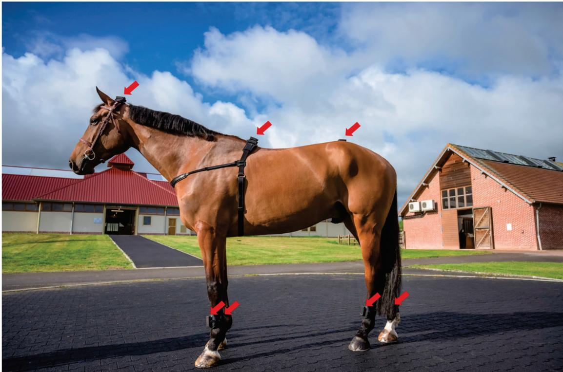
**Figure 1.** Horse equipped with EQUISYM<sup>®</sup> system, composed by sensors placed on the head, the withers, the pelvis and the four cannon bones (shown by the red arrows).
