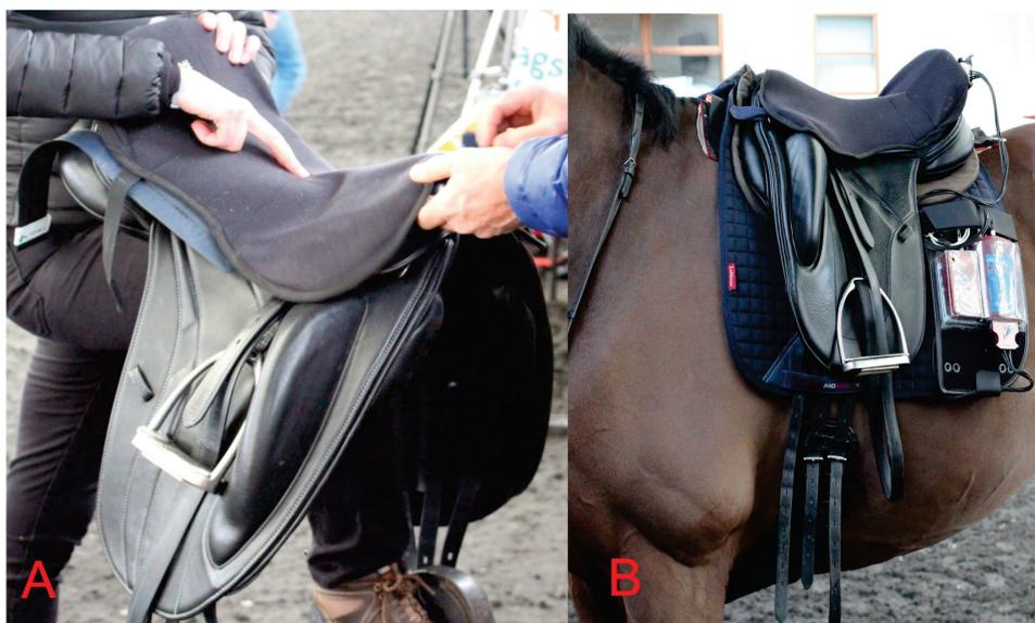
**Figure 1.** (A) Pliance force mat was positioned on top of the saddle beneath a thin cover, which was designed to prevent the force mat from displacing during locomotion. The force mat measured mean and peak pressures (kPa) with simultaneous video, and (B) the cables from the force mat were connected to a Pliance data logger, which was secured to the saddle pad.
