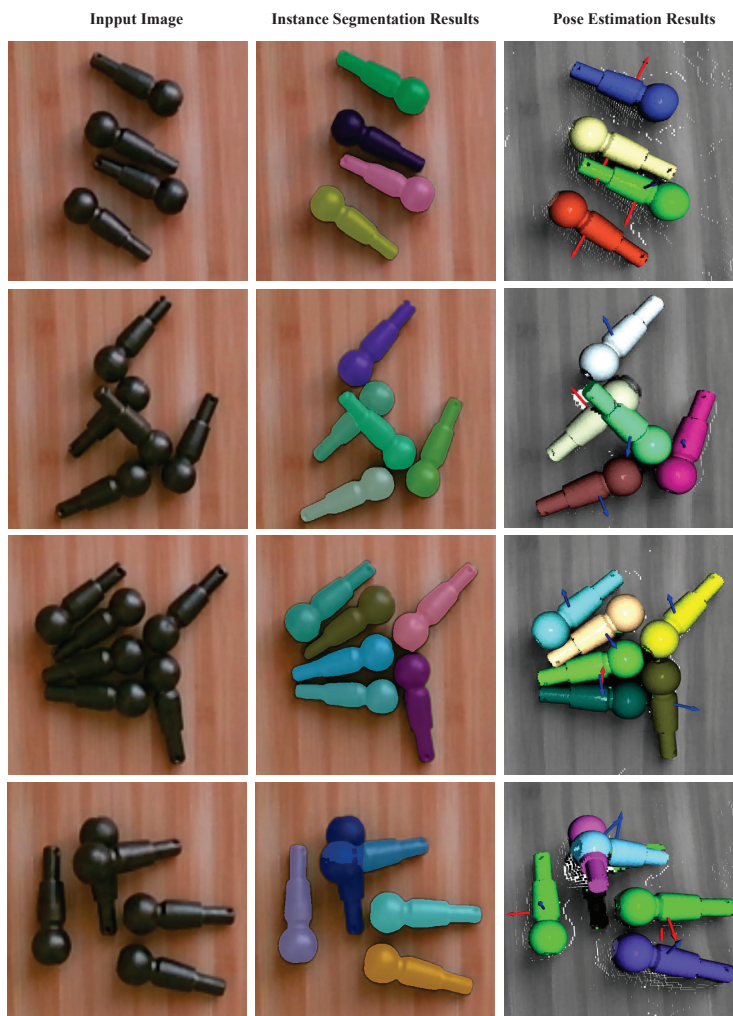
Figure 13. Qualitative results of pose estimation experiments. The three columns in the image represent, respectively, the input RGB image, the segmentation result of CAE-SAM, and the pose estimation result. The first three rows display successful matching examples, while the fourth row shows an example of an unsuccessful match.
