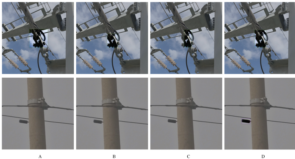
Figure 9. Visual detection results of occluded fittings under various methods. The first row shows images of a thimble obscured by steel strands, the second row shows images of a damper obscured by a cement pole. A is the U-Net, B is the U-Net combined with the DGCNN, C is the BRA-UNet, and D is the UD-Net.
