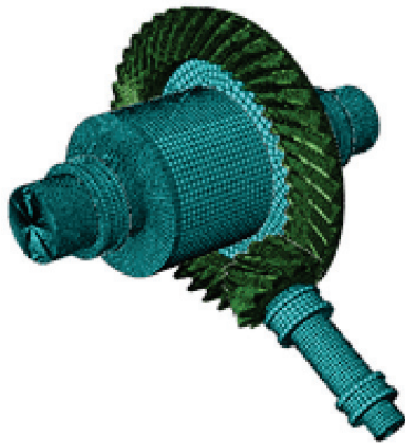
Figure 10. Finite element meshes of a spiral bevel gear system.
