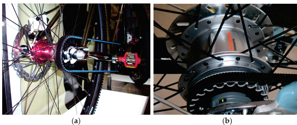
Figure 5. (a) A bicycle belt drive with horizontal fork ends and tugs for providing belt tension (courtesy of https://commons.wikimedia.org/wiki/File:Bicycle_belt_drive_1.JPG , accessed on 10 January 2025); (b) bicycle belt drive with internal-gear multispeed rear hub (courtesy of https://commons.wikimedia.org/wiki/File:Belt-drive_internal-gear_multi-speed_rear_hub.JPG , accessed on 10 January 2025).
