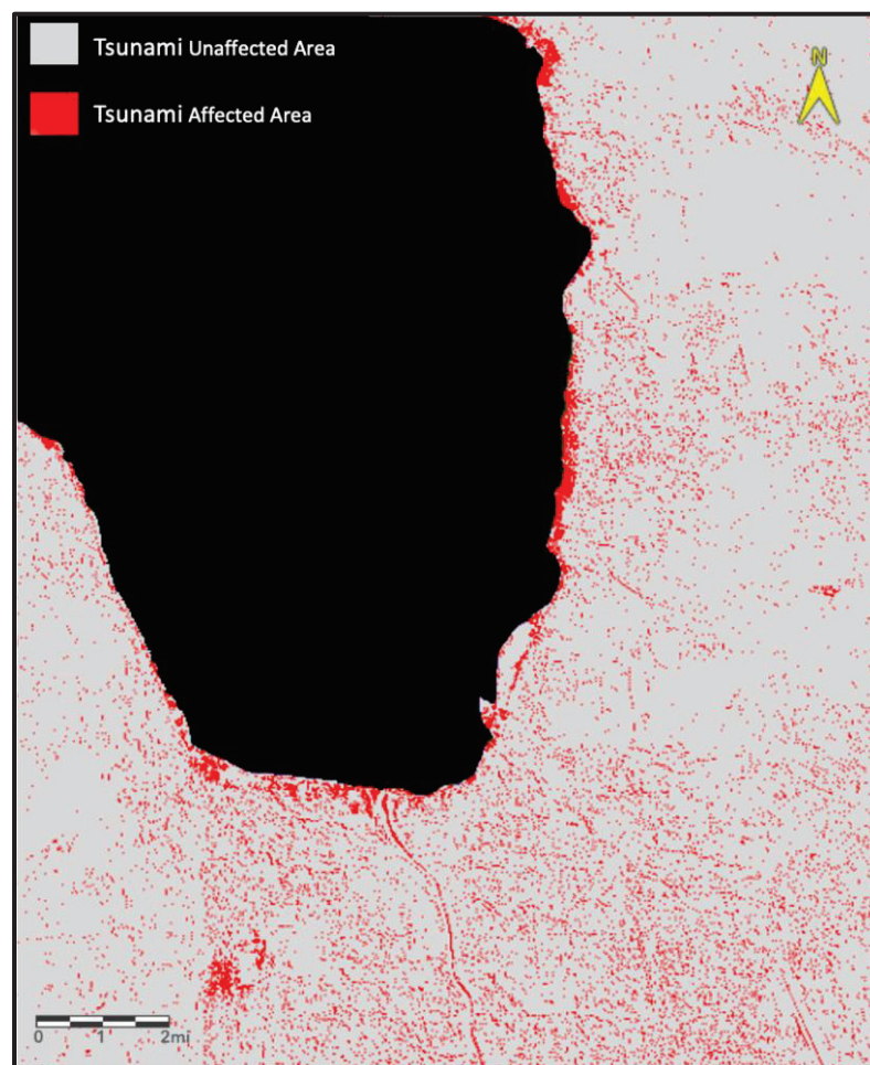
Figure 10. Final tsunami inundation map using a Decision Tree classification method, integrating the dNDVI, dNDSI, and dNDWI values obtained from pre- and post-event indices.
