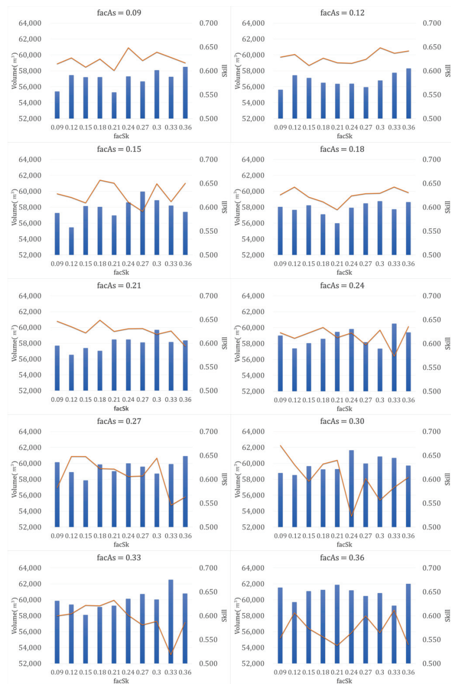
Figure 8. Changes in volume and skill values are shown in response to variations in facSk while maintaining a constant facAs.
