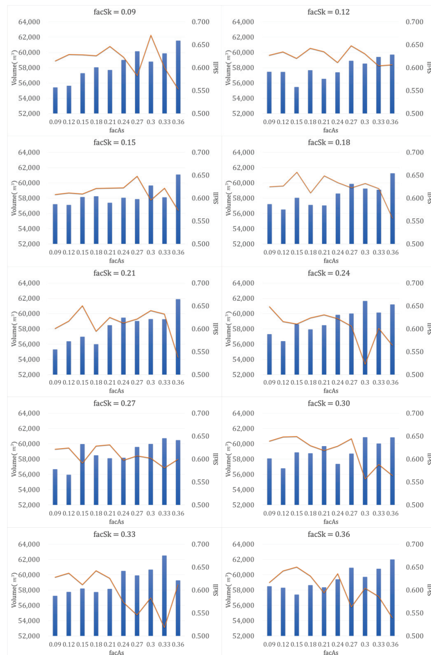
Figure 7. The variations in volume and skill values in response to changes in facAs, with a constant facSk.
