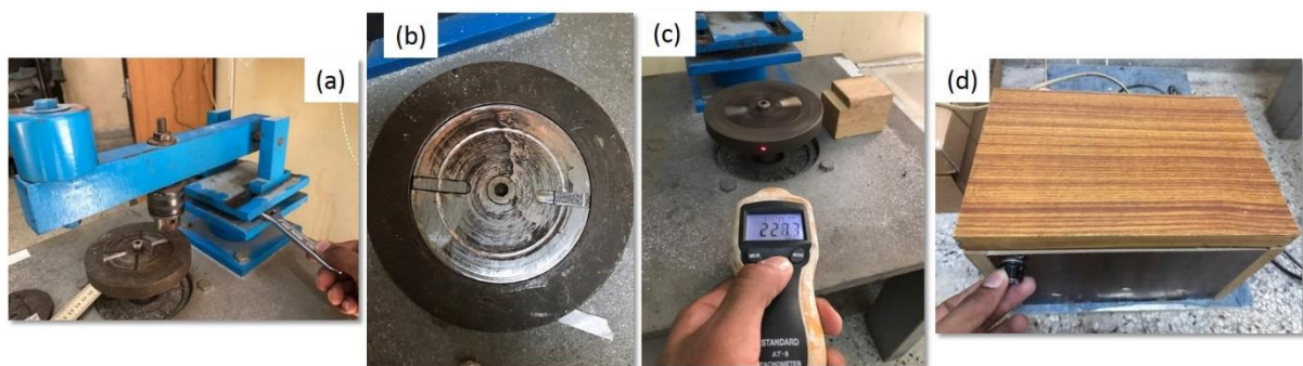
Figure 3. Execution sequence of wear testing; (a) wear testing machine, (b) fixture having two slots placed onto the disc holder is separately (c) tachometer, (d) controller box.
