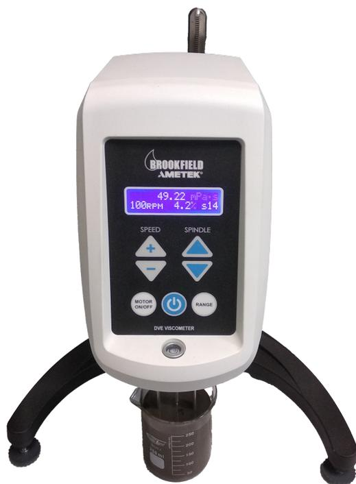
**Figure 5.** Viscosity measurement of copper ore slurry.
