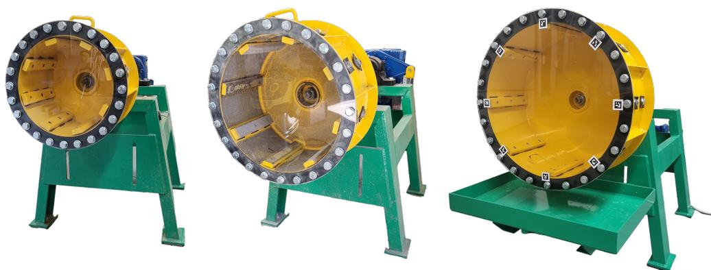
Figure 4. Ball mill with different drum sizes.
