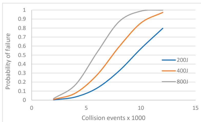
**Figure 13.** Probability of failure based on energy level the steel media is subjected to.
