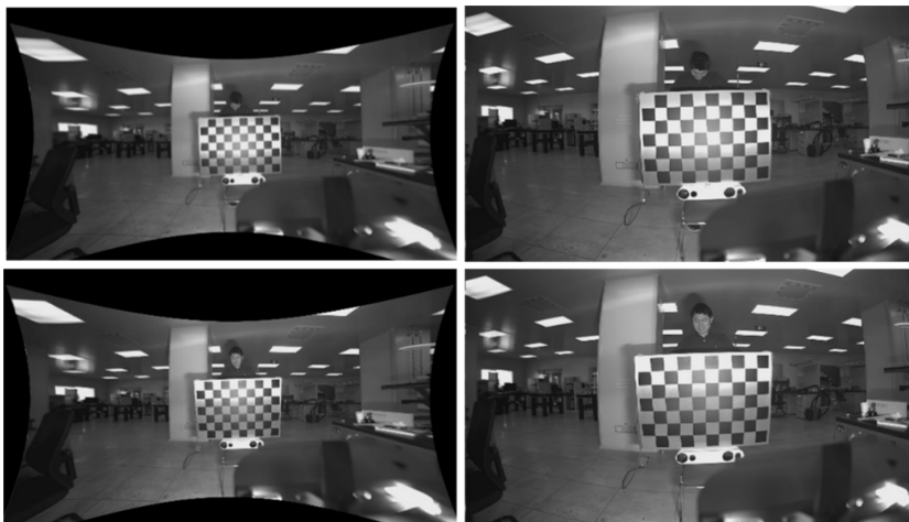
Figure 23. Aberration and correction maps for visible light camera (left lens).
