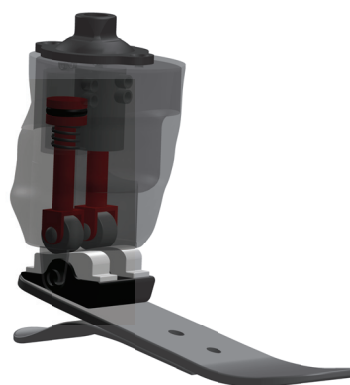
Figure 1. The new hydraulic ankle prosthesis described in [11,13]: a solid model including the main components (cams, rollers, followers, rams) and a foot consisting of two carbon fibre laminates.
