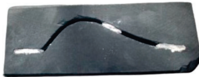
Figure 4. CNC-carved graphite template with NiTiCu wires fixed inside it, so that it can reshape and take the medial arch foot shape.
