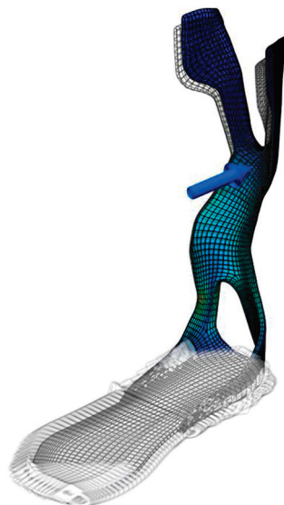
Figure 5. Finite element modeling and analysis of ankle-foot orthosis.
