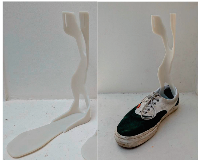
Figure 6. Three-dimensional-printed prototype of the custom-designed ankle–foot orthosis.
