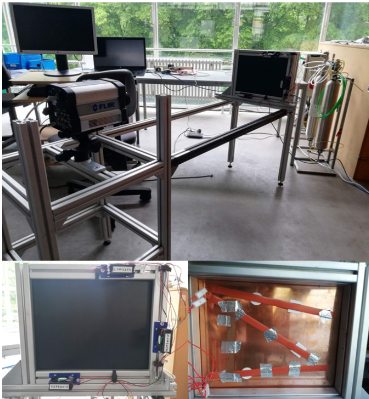
Figure 1. The physical setup is devised as a multi-mode cooling problem, depicted in the upper section. The arrangement of fans around the copper plate is illustrated in the lower left corner, while the configuration of heating strips at the back of the plate, along with randomly placed thermal insulators, is shown in the lower right corner.
