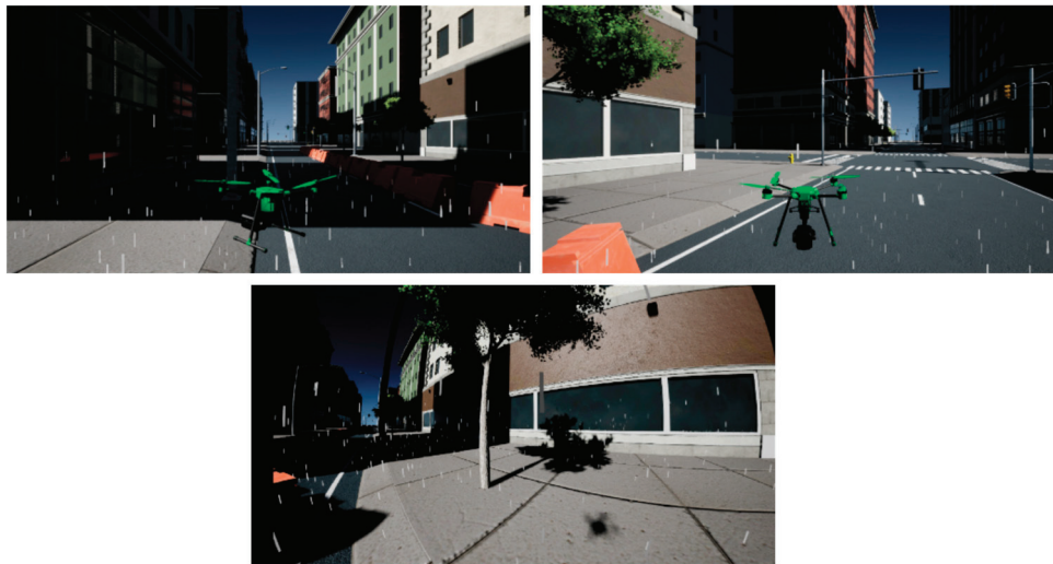
Figure 11. MATLAB simulation using the UAV Toolbox sub-figures on top show different angles of the simulated UAV and the bottom shows the feed from the fisheye image sensor.
