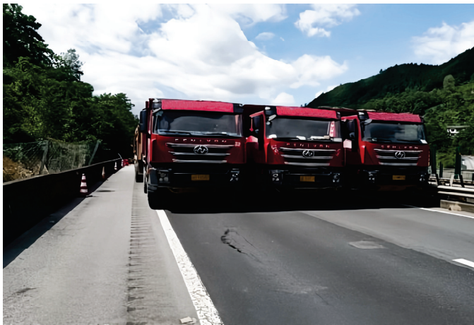
Figure 19. Photograph of the load-testing vehicle during the loading process.
