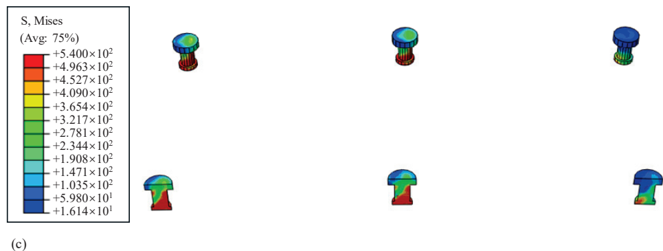
Figure 16. Specimen N-SUCS-3.1%-250: (a) Tensile damage contours of UHPC slab; (b) longitudinal stress contours of UHPC slab and steel plate; (c) stress contours of the pegs.
