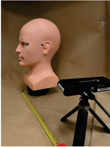
**Figure 4.** Setting scanning distance. The image shows one of the mannequin heads on the rotational base, a meter with the set distance, and the camera mounted in the tripod.
