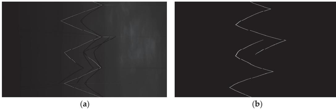
**Figure 12.** Comparison of catenary images illuminated by two types of light sources in daytime inspection: (a) white LED lamps and (b) blue stroboscopic LED lamps with band-pass optical filters.
