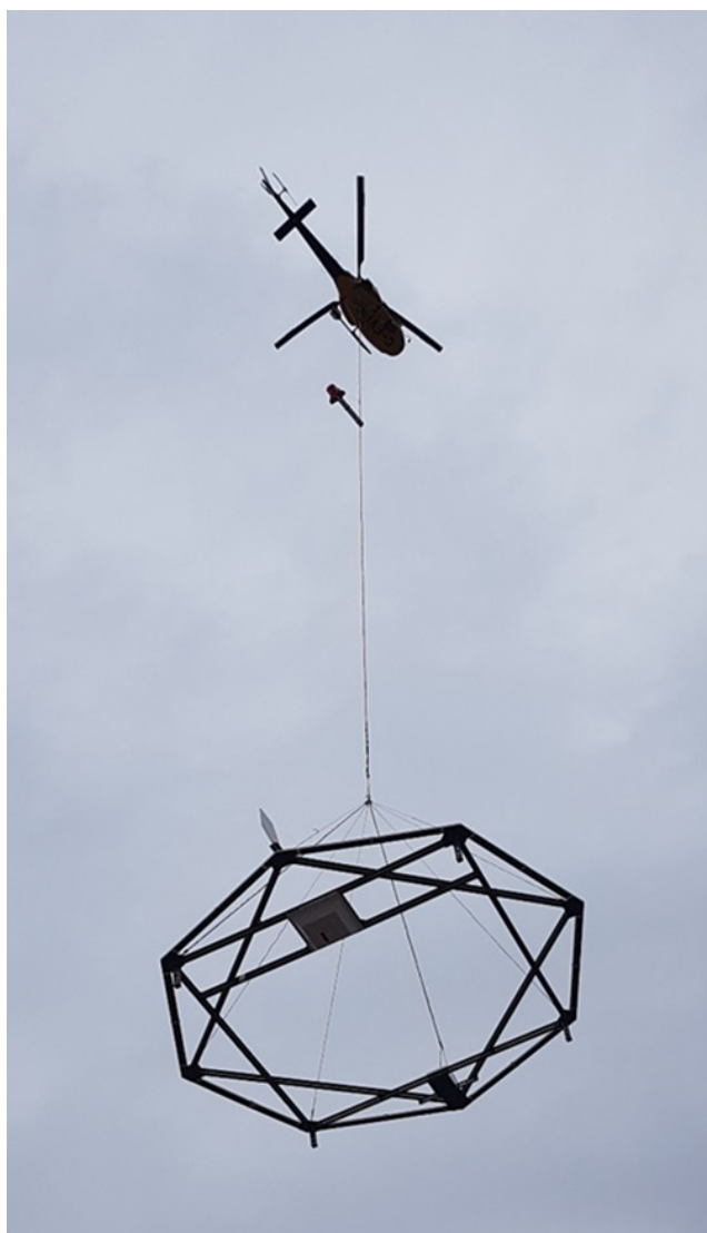
Figure 2. Example of a helicopter TDEM system (AirTEM) towed below the aircraft. The receiver is located on the same bird as the transmitter.
