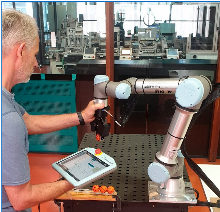
Figure 2. Programming UR5e with the teach pendant and hand guiding by a human operator.
