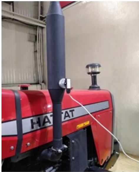
Figure 13. A view of the accelerometer placed on the exhaust.
