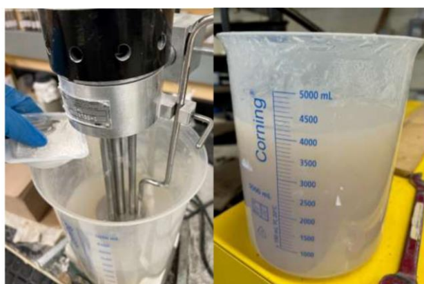
Preparation of CNC suspension using Gifford-Wood homogenizer 10 wt% CNC stock solution
