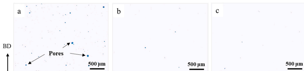
Figure 4. Cross-sectional porosity results of Hastelloy X in the building direction plane: (a) as-built, (b) HT1, and (c) HT2.
