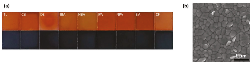
Figure 10. (a) Photographs of perovskite films fabricated using different anti-solvents before (the top brown one) and after annealing (the bottom black one) (b) Top view SEM images of the EA-processed perovskite films after annealing. Reproduced from Ref. [66] with permission from Wiley-VCH.
