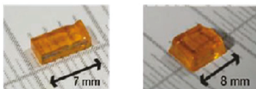
Figure 7. Photographs of the obtained CsPbBr 3 single crystals. Reprinted with permission from [101], Copyright 2016, American Chemical Society.
