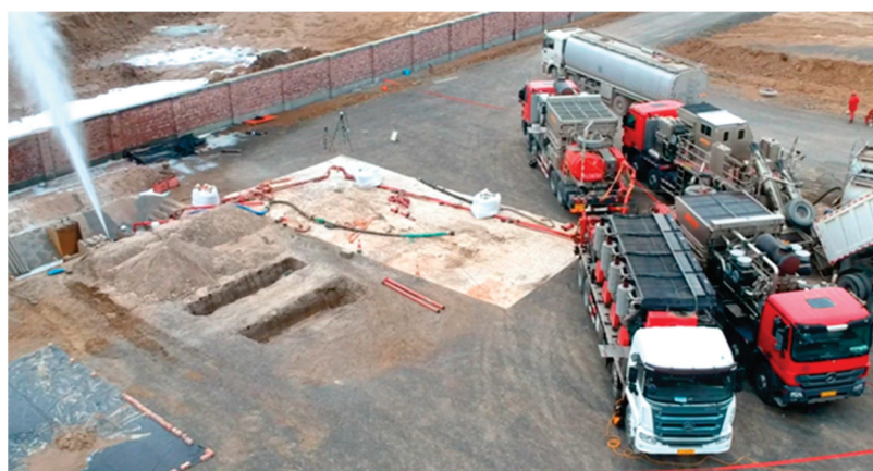
Figure 2. Field-scale perforation erosion evaluation system.
