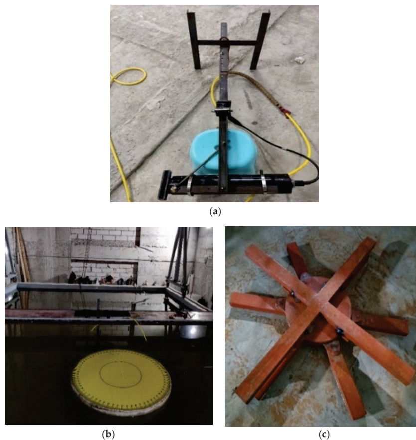
Figure 22. Experimental auxiliary device diagram. (a) Schematic of sonar fixed on angle steel frame. (b) Test tank and mobile operating platform. (c) Underwater turntable.
