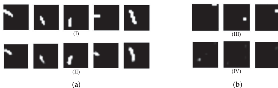
Figure 18. (a) Positive examples from MicrocrackAttentionNext (I) represents the ground truth and (II) the corresponding model prediction. (b) Failure sample (III) represents the ground truth, while (IV) shows the corresponding model prediction.
