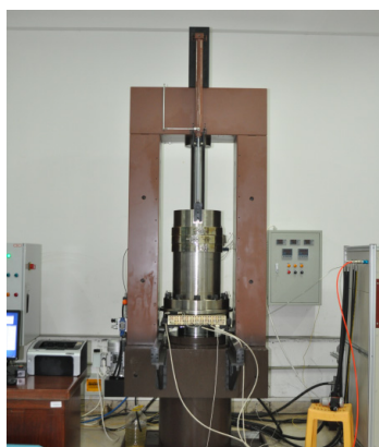
Figure 2. TFD-2000 microcomputer servo-controlled triaxial testing machine.
