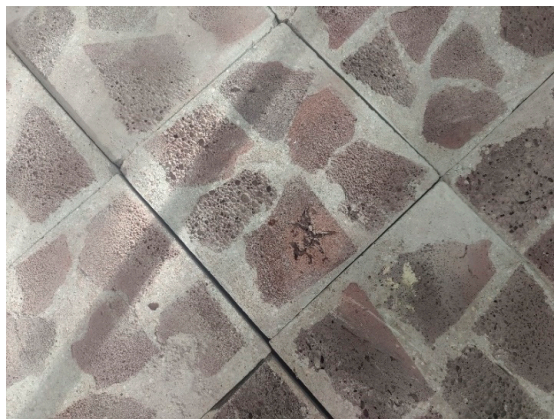
Figure 1. Slurry masonry schist specimen.
