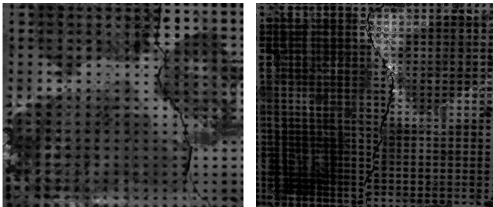
Figure 16. Damaged state of a slurry masonry schist sample.
