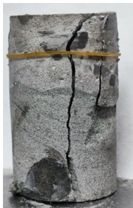
Figure 10. The damage evolution of the rock–concrete composite specimen under cyclic loads.
